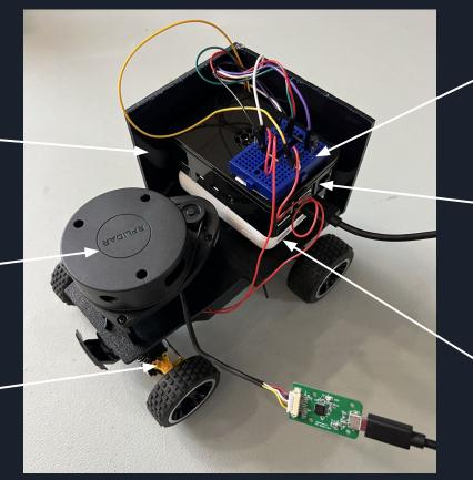
Breadboard with H-bridge turning circuit
